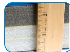
1" POLYFOAM LAYER A FIRMER 1 3/8" POLYETHYLENE LAYER
